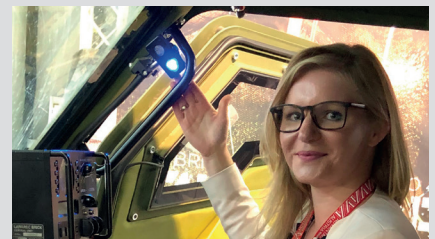
installed map-reading-light in a protected vehicle
